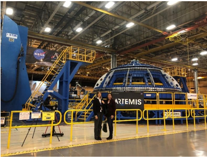
UofM Physics Alumna Michele Wilson (left) in front of the friction-stir welding fixture used to construct the dome ends on the LOX (liquid oxygen) and LH2 (liquid hydrogen) fuel tanks for the Artemis core stage at NASA's Michoud Assembly Facility in New Orleans.
