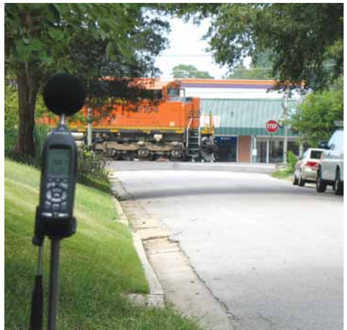
Recording Device Measures Sound Levels as Train Passes
